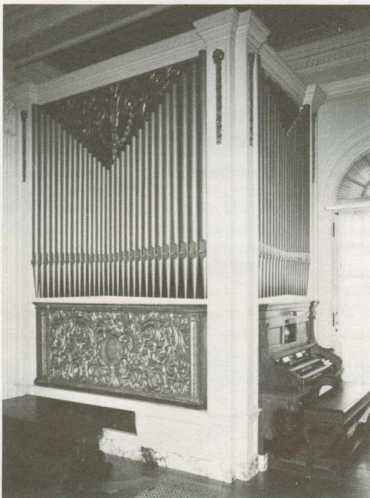
Longyear player pipe organ in Museum's music room. The two-manual console and the player mechanism with an organ roll in place are shown to the right.
